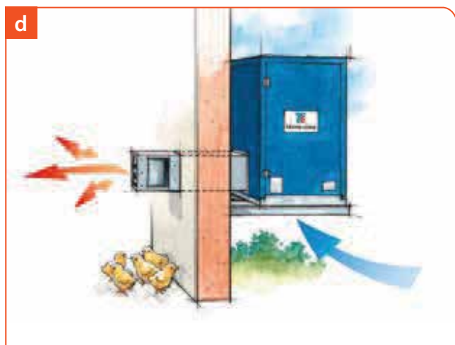
d. Outdoor, intake air from outside
