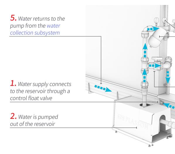
The maintenance valve remains open during normal operation
