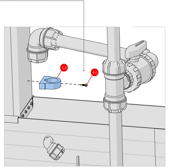
**5.** Push the pipe (32) into the pipe holder, insert one end into the reservoir channel, and attach the other end to the 90° elbow
