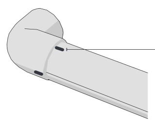
**4.** Insert the pipe into the fitting about a quarter turn from its final orientation
