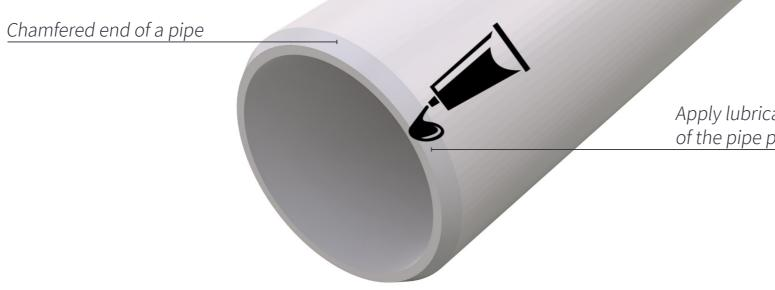
Apply lubricant to the edge of the pipe prior to insertion
