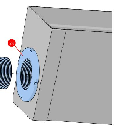
**9.** Thread the cleaning hole plug (25) into the cleaning hole sleeve
