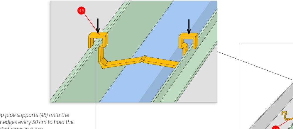
**5.** Snap pipe supports (45) onto the diffuser edges every 50 cm to hold the perforated pipes in place
