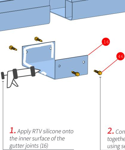
**2.** Connect two gutter sections (15) together using a gutter joint, and attach using self-drilling screws (46)
