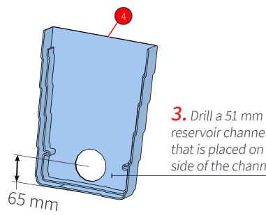
**3.** Drill a 51 mm hole in the reservoir channel end (4) that is placed on the pump side of the channel
