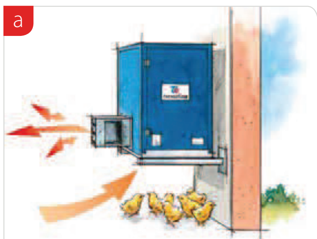
a. Indoor, intake air from inside
