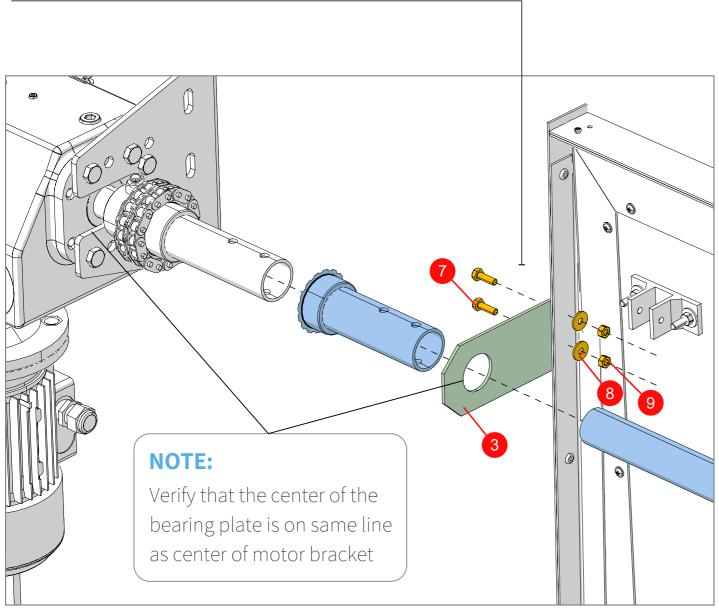
**2.** Insert the drive shaft through the sprocket (2) and into the motor coupler.
