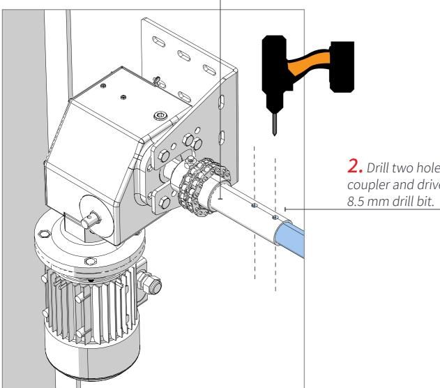
**2.** Drill two holes into the motor coupler and drive shaft using a
