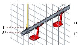
A designated suspension clip, allows raising and lowering the drinking lines. Used for Pullets and for Broilers houses.
