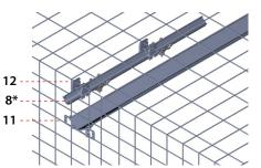
A designated clip to fix the drinking lines under the cage cieling. Used for Layers houses.
