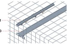
A designated clip to fix the drinking line above the cage ceiling. Used for Layers houses.
