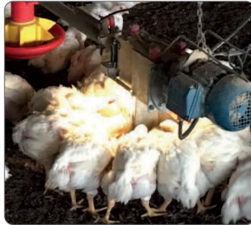
**2.** The control pan is emptied of feed quicker than the other pans on the line
