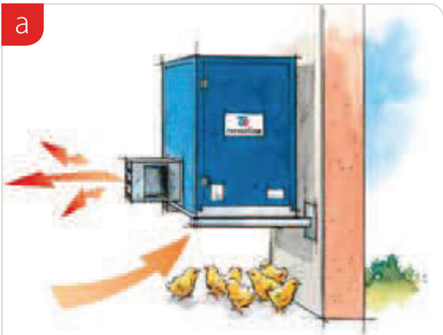
a. Indoor, intake air from inside
