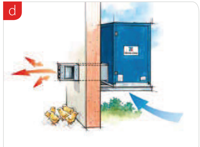
d. Outdoor, intake air from outside
