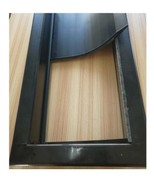
6. Install frame bar 4 to complete the main frame, and install and tighten another 4 self-drill screws as well. Please note that all frame bars should be match tightly without gap.
